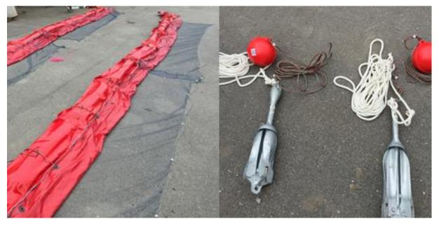
Figure 2. Litter booms with net curtains and grapnel anchors used to moor the litter boom.
