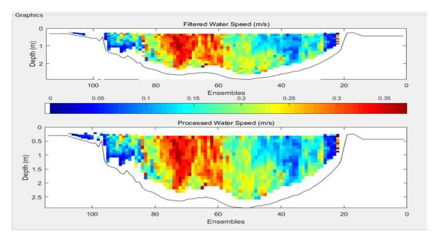
Figure 4. Example of the water flow profile at the Kerava River (Finland) that was monitored in the BLASTIC project by SYKE.
