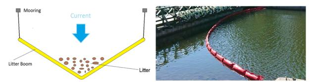
Figure 1. Set-up of the floating litter boom.
