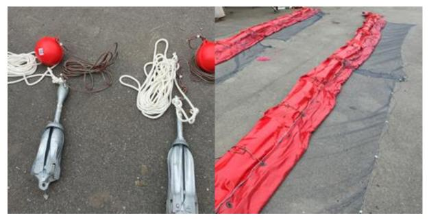
Figure 4. Grapnel anchors with marking buoys. Figure 5. Litter boom with net curtain
