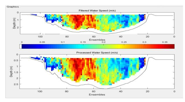
Figure 43. The river depth and water flow profile at the Kerava upstream site.
