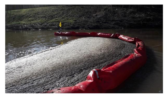
*Figure 42. Foam formed inside the boom during a 24h period (between two samplings). Photo: Outi Setälä.*
